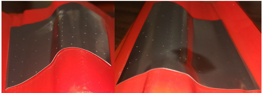
Result of Compensated Tool Surface Utilizing 3D Printing
